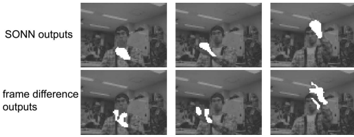
Fig. 23 Examples of blank wall problems.
