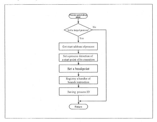
Fig. 4-3 Detection of process generation event
