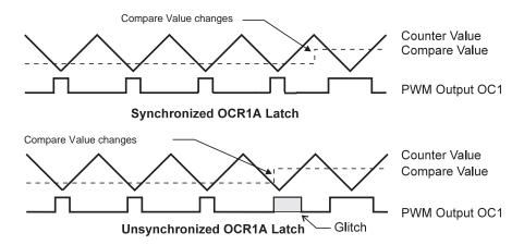
During the time between the write and the latch operation, a read from OCR1A will read the contents of the temporary location. This means that the most recently written value always will read out of OCR1A.
