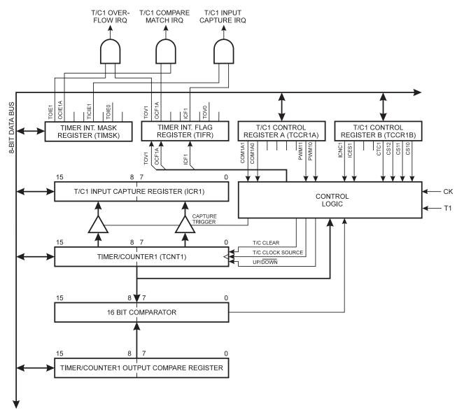
The 16-bit Timer/Counter1 can select clock source from CK, prescaled CK, or an external pin. In addition it can be stopped as described in the specification for the Timer/Counter1 Control Register - TCCR1B. The different status flags (overflow, compare match and capture event) and control signals are found in the Timer/Counter Interrupt Flag Register - TIFR. The interrupt enable/disable settings for Timer/Counter1 are found in the Timer/Counter Interrupt Mask Register - TIMSK.
