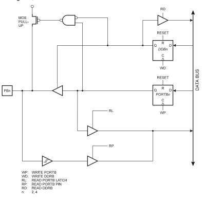
Figure 41. Port B Schematic Diagram Pin PB5
