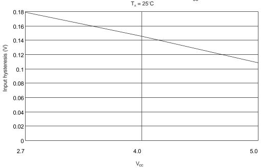
I/O PIN INPUT HYSTERESIS vs.  $V_{CC}$  $T_A = 25^{\circ}C$
