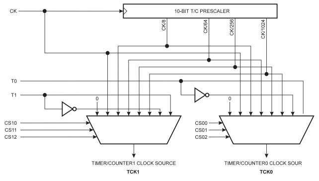
The four different prescaled selections are: CK/8, CK/64, CK/256 and CK/1024 where CK is the oscillator clock. For the two Timer/Counters, added selections as CK, external clock source and stop, can be selected as clock sources.
