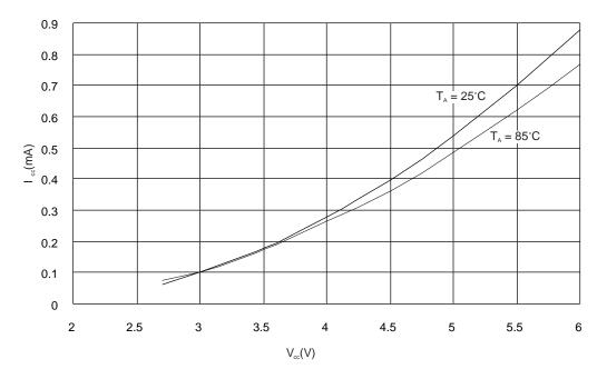
ANALOG COMPARATOR CURRENT vs. V<sub>cc</sub>
