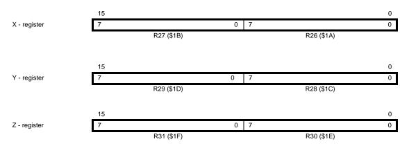
In the different addressing modes these address registers have functions as fixed displacement, automatic increment and decrement (see the descriptions for the different instructions).
