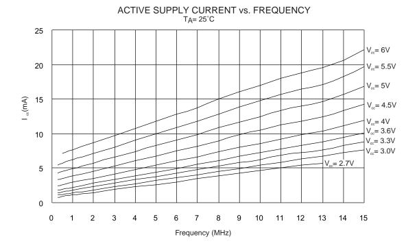
Figure 58. Active Supply Current vs. V<sub>CC</sub>
