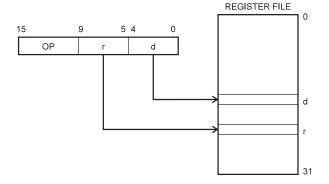
Operands are contained in register r (Rr) and d (Rd). The result is stored in register d (Rd).
