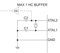
Note: When using the MCU Oscillator as a clock for an external device, an HC buffer should be connected as indicated in the figure.
