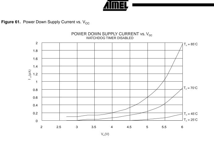
Figure 62. Power Down Supply Current vs. V<sub>CC</sub>
