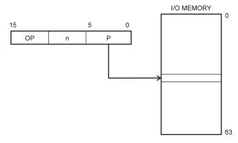
Operand address is contained in 6 bits of the instruction word. n is the destination or source register address.
