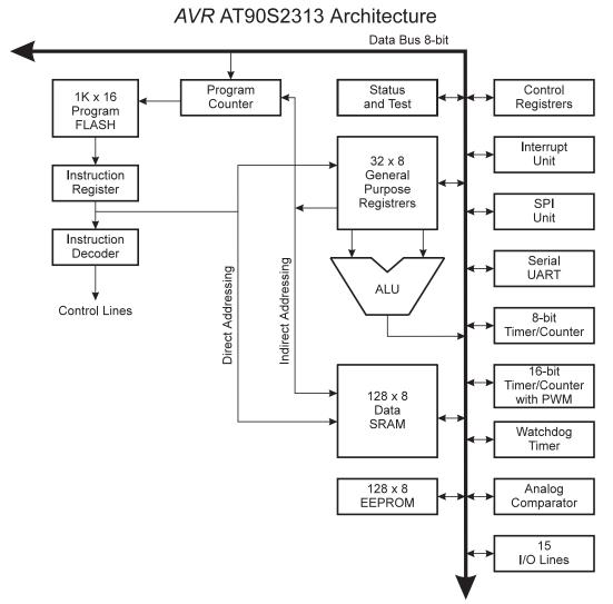
Six of the 32 registers can be used as three 16-bits indirect address register pointers for Data Space addressing - enabling efficient address calculations. One of the three address pointers is also used as the address pointer for the constant table look up function. These added function registers are the 16-bits X-register, Y-register and Z-register.
