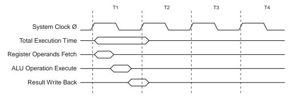
The internal data SRAM access is performed in two System Clock cycles as described in Figure 22.
