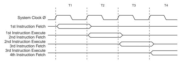
Figure 21 shows the internal timing concept for the register file. In a single clock cycle an ALU operation using two register operands is executed, and the result is stored back to the destination register.
