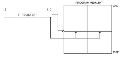
Constant byte address is specified by the Z-register contents. The 15 MSBs select word address (0 - 1K), the LSB selects low byte if cleared (LSB = 0) or high byte if set (LSB = 1).
